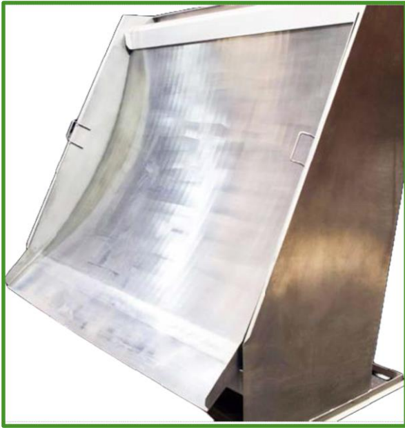
Sieve Bend Assembly with Housing
