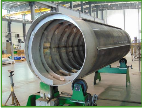
Rotary Drum for Food Processing Plant
